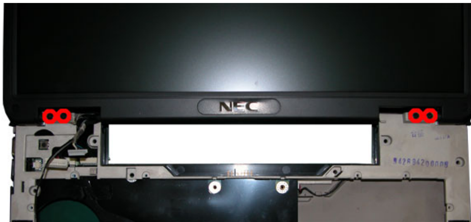
Fig. 24 Releasing the LCD Hinges
